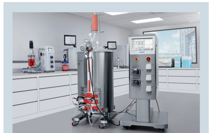
Fig. 7: The new BioFlo 720 bioreactor control system with 250 L SUB.
