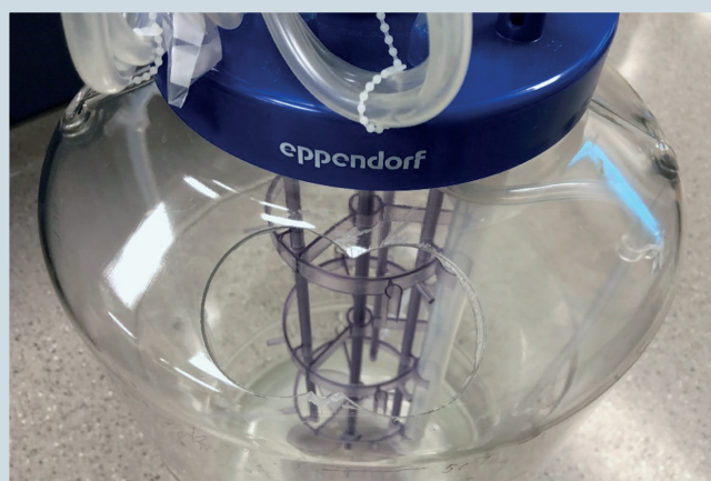
Fig. 3: The modified BioBLU 50c Single-Use Vessel.
